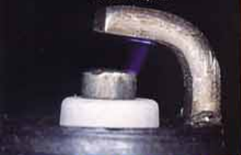
Stock Spark 13 mj spark energy, fixed at 3,500 rpm
